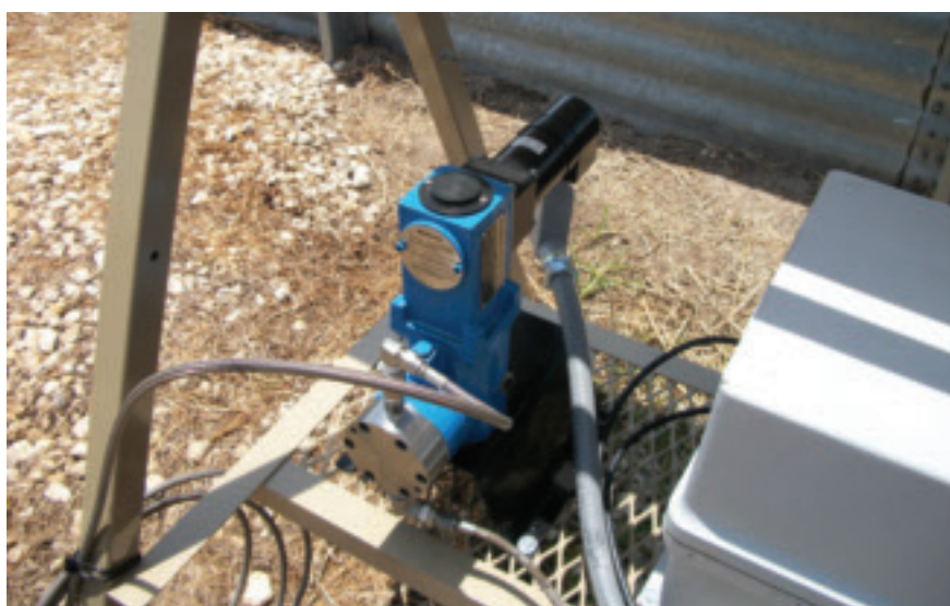
Figure 4. The iChem Solar Chemical Injection System provides accurate injection rates at well pressures up to 1,200 psi.
